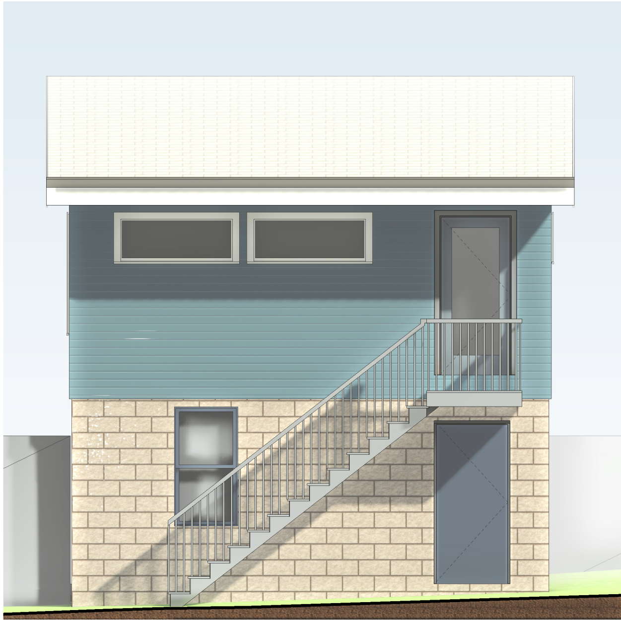
① Garage Elevation-South 1/4" = 1'-0"
